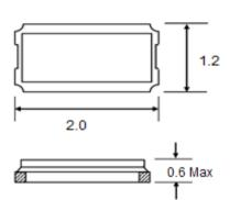
SMD Ceramic type for high population assembly Ultra light weight and thin package High stable with vacuum sealing **RoHS Complaint**
